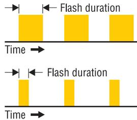
NS-600 automatically adjusts flash duration for ultra high speed and features selectable flash duration for sharper images at low speed.
